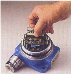
Plug-in circuit boards make maintenance quick and easy.
