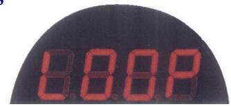
*Intellisense® LED displays "real word" messages in alpha and/or numeric symbols - enabling the operator to interpret the message immediately, without referring to a reference source.*
