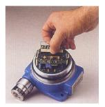
Plug-in circuit boards make maintenance quick and easy.
